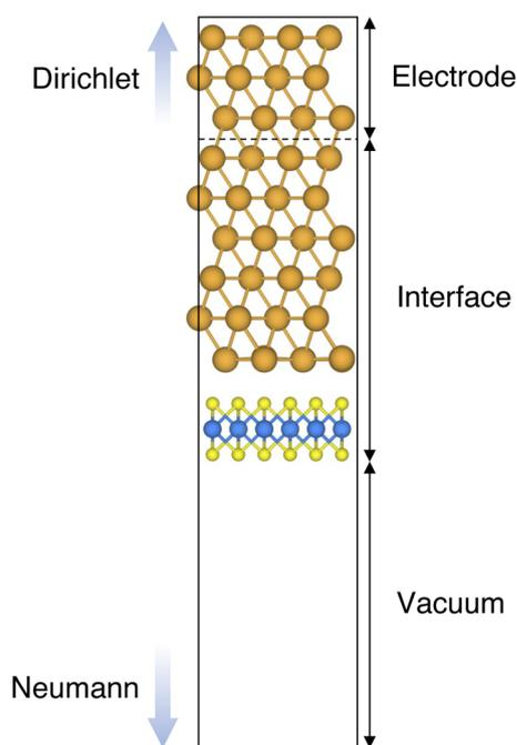
Fig. 1 Representative example of the Au/MoS<sub>2</sub> interface, modelled with the Green's function surface approach. The system can be divided into three parts: (1) the electrode (to which Dirichlet boundary conditions were applied), (2) the central part, consisting of 6 atomic layers of Au coupled with single-layer MoS<sub>2</sub>, and (3) the vacuum region, to which Neumann boundary conditions were applied.
