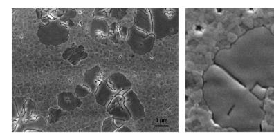
Fig. 4 SEM pictures of the 3D/2D bilayer.
