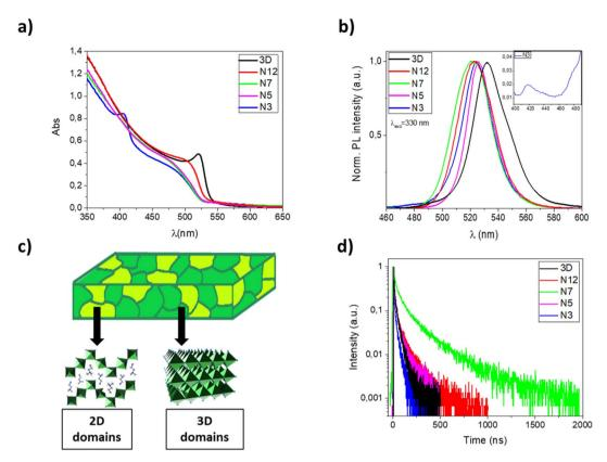
Fig. 1 (a) UV-vis absorption spectra of 3D, N12, N7, N5 and N3 thin films on glass substrates; (b) PL spectra of 3D, N12, N7, N5 and N3 thin films on glass substrates; (c) schematic of the 2D–3D perovskite thin films with domains at different dimensionality; (d) PL decay of 3D ( $\lambda_{em}$  532 nm), N12 ( $\lambda_{em}$  523 nm), N7 ( $\lambda_{em}$  520 nm), N5 ( $\lambda_{em}$  526 nm) and N3 ( $\lambda_{em}$  524 nm) thin films on glass substrates.
