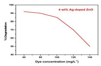
Fig. 10 Effect of concentration the degradation of dye catalysed by the 4 wt% Aq-doped ZnO NPs.
