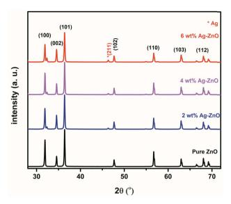
Fig. 3 XRD patterns of pure and Aq-doped ZnO NPs.
