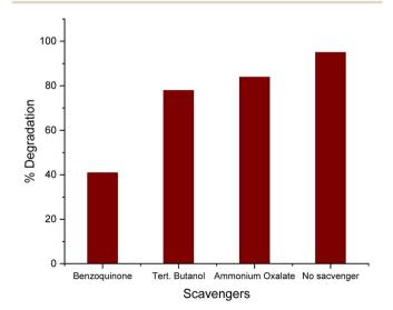
Fig. 13 Role of radical scavengers in the photodegradation of MG dye.
