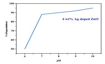
Fig. 11 Effect of pH on the 4 wt% Ag-doped ZnO NPs.
