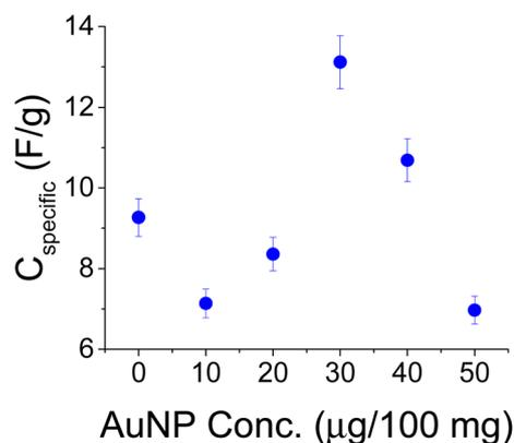
Fig. 8 Specific capacitance values derived from  $C$ - $V$  data for the CAB binder and 1 M  $\text{NaCl}$  electrolyte. A similar trend is obtained with  $C$ - $D$  data. The concentration of AuNPs in  $\mu\text{g}$  is referenced to 100 mg of AC in the batch.
