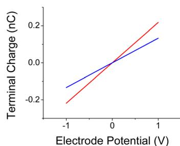
Fig. 16 Change in electrode charge as a function of the bias,  $V_{in}$ . Blue line: graphite-like electrode without any colloid; red line: graphite-like electrode with colloids on its surface. The cell capacitance is the slope of the linear  $Q-V$  curve.
