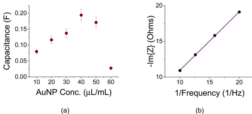
Fig. 6 (a) Capacitance values derived from EIS curves. The concentration of the AuNPs is in  $\mu\text{L}$  per 1 mL of solvent. (b) The slope of the linear curve for the sample exhibiting capacitance maxima at  $40 \mu\text{L mL}^{-1}$  of AuNPs is proportional to  $1/C_{\text{diff}}$ . The electrolyte was 1 M of  $\text{Na}_2\text{SO}_4$ .
