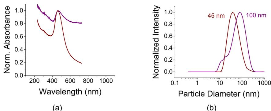
**Fig. 1** (a) Absorbance (normalized such that the peak equals unity) for ligand-coated, small size (wine color) and aggregates (purple color) of AuNPs. Both were suspended in water. The plasmonic absorption is clearly seen; the aggregate peak is a bit red-shifted and broader compared to the small particles' peak. The increase in absorption towards the UV spectrum is attributed to increased scattering. (b) The corresponding DLS data show the two particle sizes used in the experiments.
