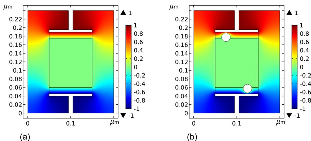
Fig. 14 Potential distribution for  $V_{in} = 1 \text{ V}$ . The neutral region indeed has a constant potential (zero in this case) and the presence of the metallic colloid alters the potential lines. (a) No colloid. (b) With 10 nm colloids. The thermal legend is in units of Volts.
