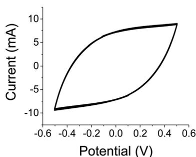
Fig. 12 125  $C$ - $V$  scans for 30  $\mu\text{g}$  of AuNPs per 200 mg of AC sample in 1 M  $\text{Na}_2\text{SO}_4$  at a rate of 50  $\text{mV s}^{-1}$  exhibited <2% change between the first and last scan.
