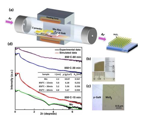
Fig. 1 (a) Schematic illustration of the CVD setup. (b) Photograph image of the  $MoS_2$  film deposited on 1 cm  $\times$  1 cm p-GaN. (c) Optical image of the large-area patterned  $MoS_2$  film grown on p-GaN through a shadow mask, taken at  $20\times$  magnification. (d) X-ray reflectivity curve of the asgrown Mo and  $MoS_2$  films deposited on p-GaN at 850 °C – 15 min, 850 °C – 30 min and 850 °C – 60 min.
