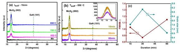
Fig. 4 (a) HR-XRD spectra of the MoS<sub>2</sub> films grown at different temperatures of 650 °C, 750 °C, and 850 °C for 15 min. (b) HR-XRD patterns of the 850 °C sample grown for different durations. (c) Full width at half maximum (FWHM) of the main XRD peak and the corresponding grain sizes of 850 °C sample as a function of sulfurization duration.
