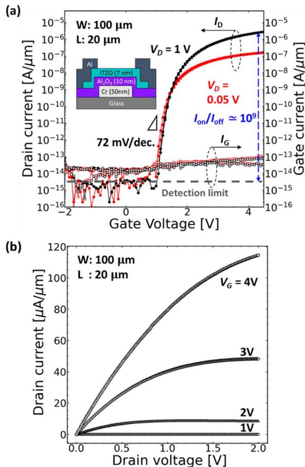
Fig. 6 (a)  $I_D$ – $V_G$  and (b)  $I_D$ – $V_D$  characteristics of the Al<sub>2</sub>O<sub>3</sub> TFT.
