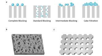
Fig. 1 Schematics of pore blocking mechanisms and membrane structures in use. (a) Most commonly recognized four different pore blocking mechanisms. (b and c) Schematic images of the membrane structure for the (b) commercial filter and (c) ultra-thin nanopore membrane (NUTS).
