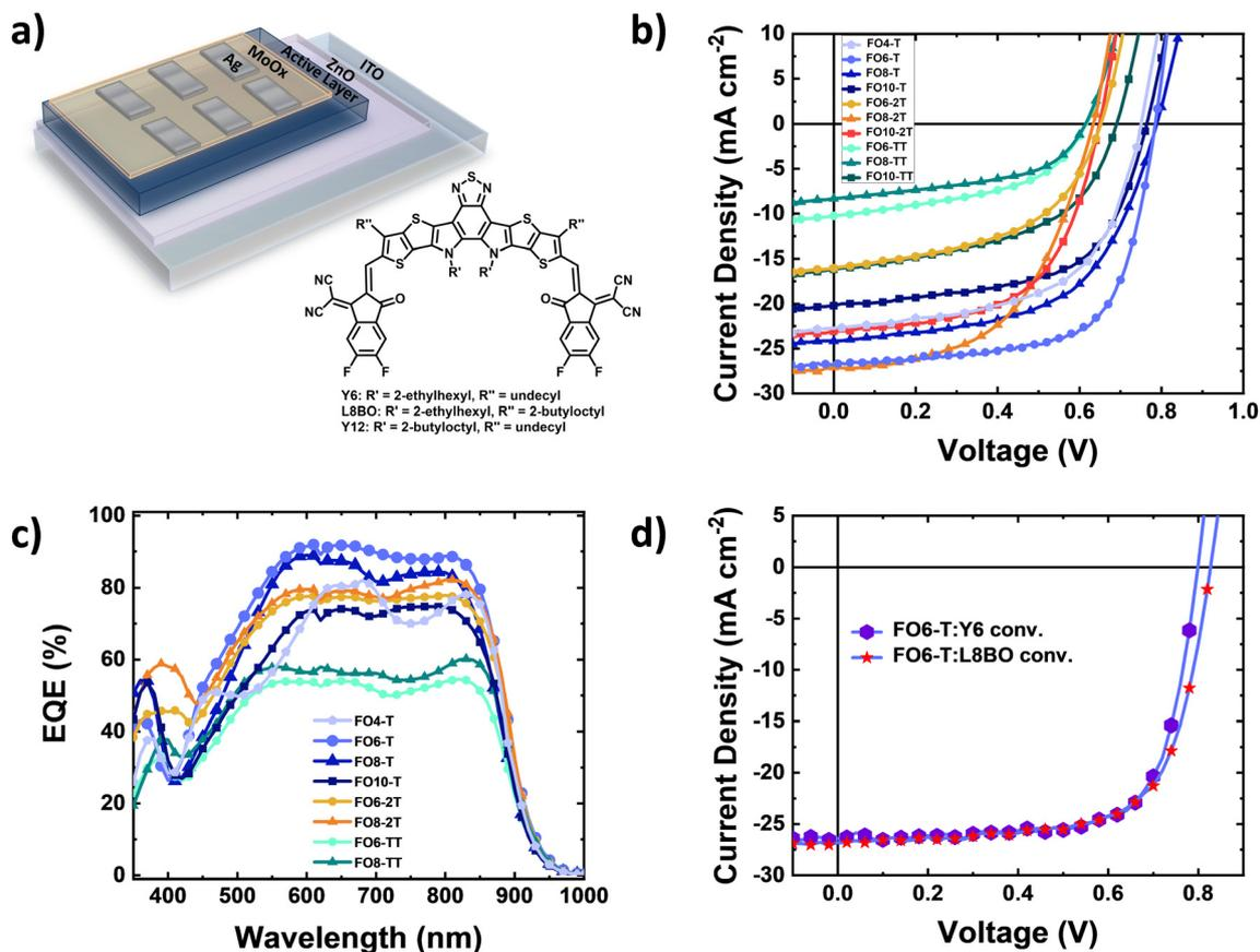
Fig. 2 (a) Device architecture of the solar cells (inverted structure) and molecular structure of the NFAs, (b)  $J$ - $V$  curves of devices under AM1.5G illumination, (c) EQE spectra of the OPV devices and (d)  $J$ - $V$  curves for devices with conventional structure L8BO and Y6 as acceptors under AM1.5G illumination.
