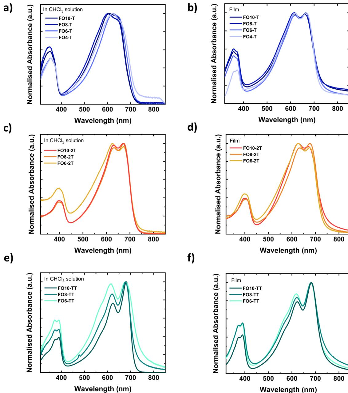
Fig. 1 UV-vis absorption spectra of polymers in solution in  $\text{CHCl}_3$  (a) FOR-T polymers, (c) FOR-2T polymers, and (e) FOR-TT polymers, and in thin film (b) FOR-T polymers, (d) FOR-2T polymers and (f) FOR-TT polymers. The solutions were prepared at a  $5 \mu\text{M}$  concentration and thin films were prepared from a  $10 \text{ mg mL}^{-1}$  solution and spin coated on glass slides.
