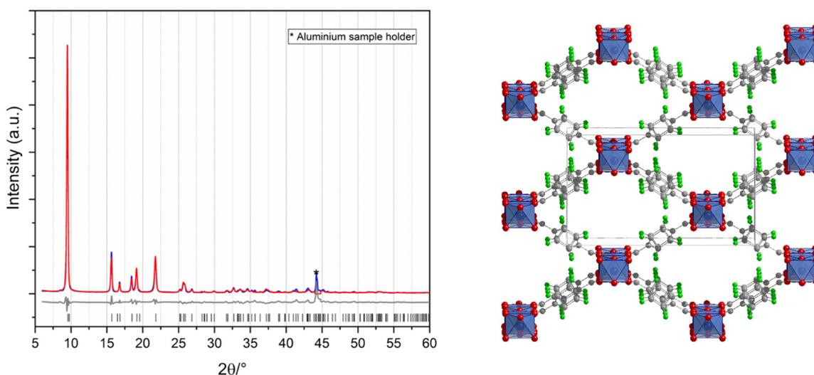
Fig. 1 Left: Rietveld refinement of F<sub>4</sub>-MIL-53(Al). The experimental PXRD pattern is shown in blue, the calculated in red and the difference (experimental – calculated) is given in grey. The allowed reflection positions are given in black. Right: Crystal structure of F<sub>4</sub>-MIL-53(Al). Colour code: aluminium (blue), carbon (grey), oxygen (red) and fluorine (green).
