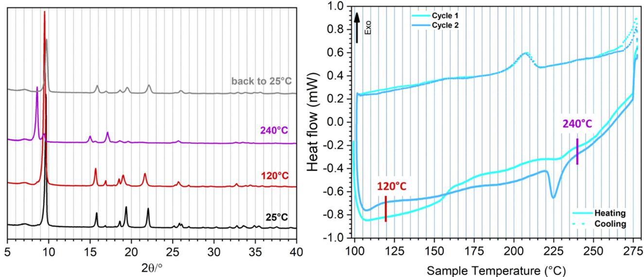
Fig. 3 VT-XRPD patterns of  $\text{F}_4\text{-MIL-53(Al)}$  at room temperature (25 °C – black), before the phase transition (120 °C red), after the phase transition (240 °C purple) and after returning to the room temperature (25 °C – light grey) (left). DSC profile of  $\text{F}_4\text{-MIL-53(Al)}$  (right): first cycle (cyan) and second cycle (light blue). Full and dotted curves refer to the heating and cooling cycles respectively (right).
