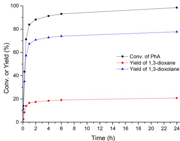
**Fig. 4** Yield/conversion & time plots for the acetalization reaction of phenylacetaldehyde with glycerol using UiO-66-15 as a catalyst. Reaction conditions: PhA – 2 mmol; glycerol – 4 mmol; catalyst – 10 mg (1.5 mol% Zr); reflux of toluene (6 ml), Dean–Stark.
