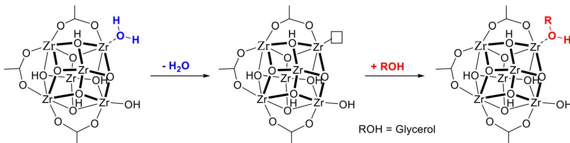
Fig. 5 Removal of polarized H<sub>2</sub>O molecules during UiO-66 dehydration and formation of novel Brønsted-induced acid sites upon glycerol adsorption.
