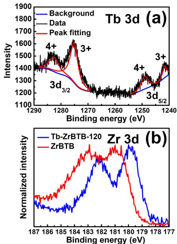
Fig. 5 XPS spectra of (a) Tb-ZrBTB-120 in the region of Tb 3d, and (b) Tb-ZrBTB-120 and ZrBTB in the Zr 3d region.
