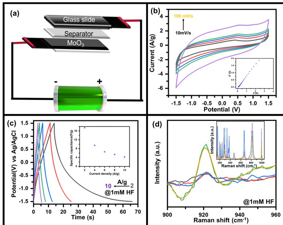
Fig. 4 (a) Schematic diagram of as-fabricated  $\text{MoO}_3//\text{AC}$  supercapacitor device, (b) CV curves measured at scan rates of 10 to  $100 \text{ mV s}^{-1}$  along with the corresponding EIS plot ( $\text{ESI}^\dagger$ ), (c) GCD plots at  $2 \text{ A g}^{-1}$  to  $10 \text{ A g}^{-1}$  along with variation of specific capacitance as a function of current density (inset) and (d) *in situ* Raman spectra of asymmetric supercapacitor device during the charging and discharging process.
