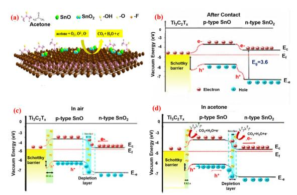
Fig. 8 Schematic illustration of the band diagram of the p-n heterojunction and the combination of the  $SnO-SnO_2/Ti_3C_2T_x$  sensor. Adopted with permission from ref. 139. Copyright 2020 Material Science Technology.
