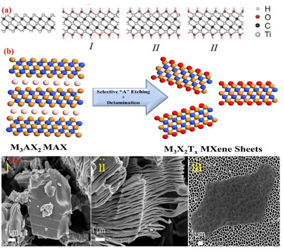
Fig. 4 (a) Configuration of the OH groups: (i)  $Ti_3C_2(OH)_2$ , (ii)  $Ti_3C_2(OH)_2$ . Adopted with permission from ref. 73. Copyright 2012, Computational and Theoretical Chemistry, Elsevier. (b) Schematic illustration of the MXene synthesis process from the MAX phase. (ii) MAX phase, (iii) Multilayer MXene, and (iii) MXene assembled flakes in a colloidal solution. Adopted with permission from ref. 62. Copyright 2017, American Chemical Society.
