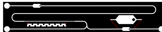
Fig. 3 Design of the microfluidic channels for mixing of M1 particles (right bottom inlet) and Fmoc-pY-OEt.TBA (left bottom inlet) solutions in chloroform and fluorescence analyses before and after mixing. Zoomed-in areas show the square serpentine passive mixer and a 1 mm large fluorescence acquisition chamber (not to scale).
