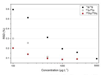
Fig. 1 Isotope ratio precision of  $^{11}B/^{10}B$ ,  $^{87}Sr/^{86}Sr$  and  $^{208}Pb/^{206}Pb$ . expressed as RSD (%), for an acquisition time of 10 s per run (M) and M = 20, obtained for different elemental mass concentrations. The data shown are from the measurement of a mixture in which B. Sr. and Pb were detected simultaneously.
