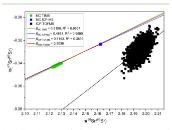
Fig. 4 Three-isotope plot for Sr from measurements over several hours of NIST SRM 987 using ICP-TOFMS (integration time 0.5 s, M = 2000), MC TIMS (integration time 24 s, M=443) and MC ICP-MS (integration time 42 s, M = 238). Solid lines represent experimentally determined slopes ( $\beta_{instrument}$ ) and predicted mass dependent fractionation line ( $eta_{ ext{theo-Russell}}$ ). All data points were taken from measurements of pure NIST SRM987 single-element solution.
