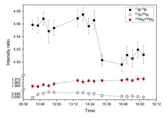
Fig. 2 Long-term stability of  $^{11}$ B/ $^{10}$ B,  $^{87}$ Sr/ $^{86}$ Sr and  $^{208}$ Pb/ $^{206}$ Pb isotope ratios over eight hours for 15 discontinuous measurements of NIST SRM 951a, NIST SRM 987 and NIST SRM 981. Error bars correspond to 2 s (acquisition time of 10 s, M=20). The data shown are from the measurement of a mixture in which B, Sr, and Pb were detected simultaneously.
