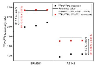
Fig. 6  $^{208}$ Pb/ $^{206}$ Pb intensity ratios and absolute  $^{208}$ Pb/ $^{206}$ Pb isotope ratios (internal inter-elemental IIF correction using Tl) for three measurements of NIST SRM 981 and ERM-AE142. Error bars (smaller than symbols) correspond to 2 s (acquisition time of 10 s, M=20) and are smaller than the symbols. The data shown are from the measurement of a mixture in which B, Sr, Tl and Pb were detected simultaneously.
