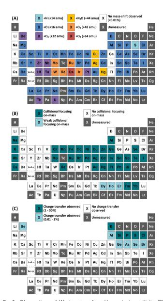
Fig. 2 Observations of (A) atom transfer with greatest sensitivity. (B) on-mass collisional focusing, and (C) asymmetric charge transfer reactions using N2O reaction gas.
