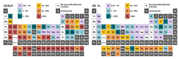
Fig. 1 Comparison of maximum achieved sensitivity (relative to standard mode) for mass-shift determinations (by atom transfer) using (A) N<sub>2</sub>O and (B) O<sub>2</sub> reaction gases.
