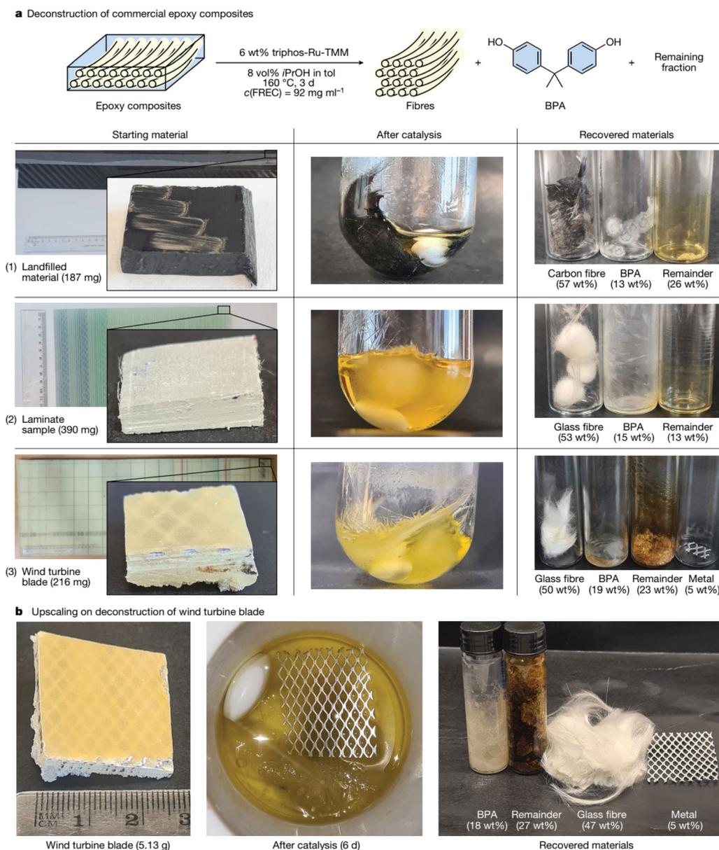
**Fig. 8** Recovery of BPA and fibers from commercial epoxy composites using Ru catalysis. (a) Scope of the composite samples subjected to catalysis (both length and width of composite pieces 1, 2 and 3: 1.0–1.5 cm) and (b) upscaling of deconstruction conditions for end-of-life WTBs. Reproduced from ref. 83 with permission from Springer Nature, copyright [2023].
