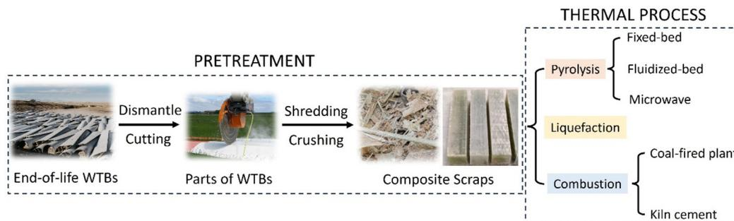
Fig. 5 Thermal recycling processes of end-of-life WTBs.
