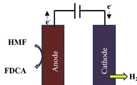
Fig. 27 Schematic illustration of HMFOR and HER. Modified from ref. 268 with permission from Elsevier, copyright 2022.
