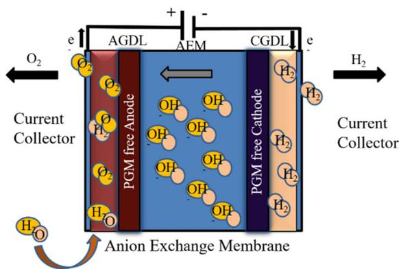
Fig. 12 Working principle of an AEM electrolysis cell.
