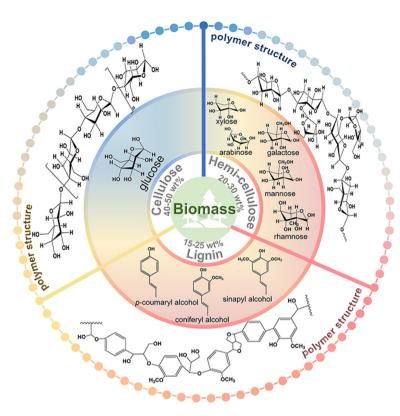
Fig. 1 The polymer structures and depolymerized monomers/monomeric units of the three major components of biomass.
