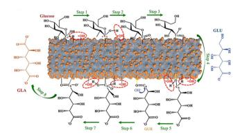
**Fig. 4** Possible reaction pathway from glucose to glucaric acid over the Pt/def-TiO<sub>2</sub> photoanode. Adapted from ref. 38 with permission from Springer Nature, copyright 2023.
