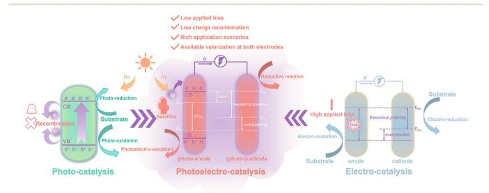
Fig. 2 Comparison of photo-, electro-, and photoelectro-catalysis.  $E_{FP}$  and  $E_{FN}$  are the quasi Fermi levels of holes and electrons, respectively;  $E_{Ox}$  and  $E_{Re}$  are the oxidative and reductive potentials of the substrate, respectively.
