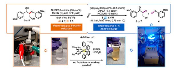
Fig. 11 Schematic for the one-pot electrocatalytic oxidation-reductive cleavage of  $\beta$ -O-4. Adapted from ref. 83 with permission from the American Chemical Society, copyright 2017.
