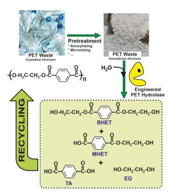
Fig. 8 Schematic representation of a circular chemistry process for recovery and reuse of polyethylenepterephtalate (PET), based on the enzymatic hydrolysis by means of engineered biocatalysts. 105
