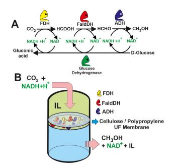
Fig. 6 (A) Scheme of a multi-enzyme system for methanol synthesis from CO<sub>2</sub> with in situ regeneration of NADH. (B) Set-up of the proposed IL-based multi-enzymatic membrane reactor for CO<sub>2</sub> transformation to methanol.80
