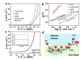
Fig. 3 (a) OER LSV curves of the bare GC electrode, commercial 20 wt% Pt/C, CoS<sub>2</sub> and IL-modified CoS<sub>2</sub> and (b) the derived Tafel plots. (c) OER LSV curves of IL-modified CoS<sub>2</sub> before and after 1000 CV tests. (d) Schematic illustration of the oxidation of water. Reproduced with permission. <sup>46</sup> Copyright 2018, the Royal Society of Chemistry.
