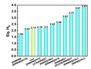
Fig. 9 Dehydrogenation yields of EDB supported by imidazoliumbased ILs. Reproduced with permission.<sup>67</sup> Copyright 2013, Elsevier.
