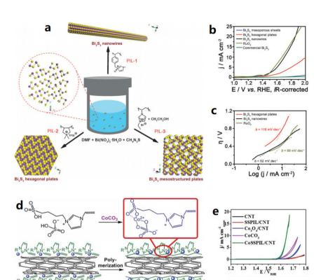
Fig. 2 (a) PILs controlled the structures of  $Bi_2S_3$ , (b) OER linear sweep voltammetry (LSV) curves of  $Bi_2S_3$  and  $RuO_2$ , (c) Tafel slope of  $Bi_2S_3$  and  $RuO_2$ . Reproduced with permission. As Copyright 2016, Wiley-VCH; (d) preparation procedure of CoSSPIL/CNT, and (e) cyclic voltammogram (CV) of CoSSPIL/CNT compared to different samples of CNT, SSPIL/CNT,  $Co_3O_4/CNT$ , and  $CoCO_3$ . Reproduced with permission. As Copyright 2018, Wiley-VCH.
