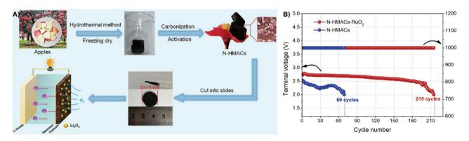
Fig. 18 (A) The synthesis strategy of N-HMACs and the construction of a Li-O<sub>2</sub> battery with an N-HMAC cathode. (B) Voltage of the terminal discharge and the cycle number. 195 Reprinted with permission. Copyright 2020, Elsevier.
