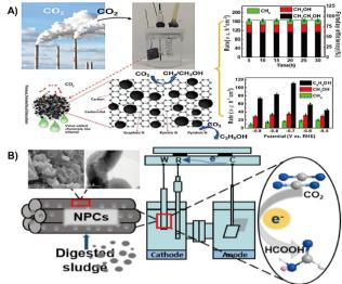
Fig. 12 (A) Municipal sludge derived carbon dots modified, N-doped biochar for the electrochemical reduction of carbon dioxide.<sup>28</sup> Reprinted with permission. Copyright 2022, Elsevier. (B) Nitrogen-doped porous carbon from digested sludge for the electrochemical reduction of carbon dioxide to formate. 135 Reprinted with permission. Copyright 2018, American Chemical Society.
