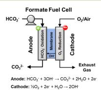
Schematic representation of a direct formate fuel cell.
