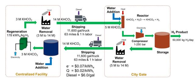
Fig. 6 Material flow diagram used for an initial cost analysis of the hybrid bicarbonate/formate cycle (electrochemical reduction of bicarbonate coupled with catalytic oxidation of formate to bicarbonate) for a regional refueling depot use case.
