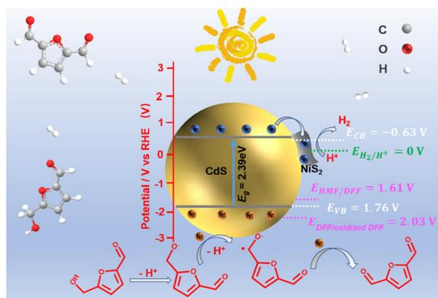
**Scheme 1** Schematic illustration of the determined CB and VB edges of NiS<sub>2</sub>/CdS and oxidizing potential.
