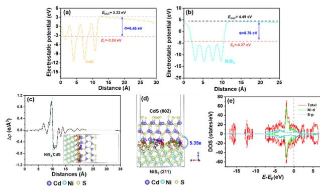
**Fig. 4** Theoretical work functions of CdS (a) and NiS<sub>2</sub> (b). (c) Electron density difference (e Å<sup>-3</sup>) and (d) Bader electron transfer at the NiS<sub>2</sub>/CdS interfaces. (e) The density of states of NiS<sub>2</sub>.
