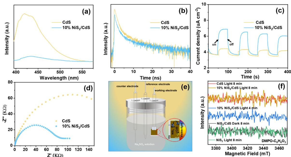
**Fig. 5** (a) PL spectra, (b) TRPL decay spectra, (c) transient photocurrent responses, and (d) EIS spectra for pure CdS and 10% NiS<sub>2</sub>/CdS; (e) schematic of photochemical cell and electron flow; (f) *in situ* EPR spectra for CdS, NiS<sub>2</sub> and 10% NiS<sub>2</sub>/CdS in a mixture solution of HMF in the presence of spin-trapping agent DMPO with or without visible light irradiation.
