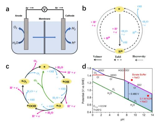
Fig. 2 (a) Schematic illustration of electrochemical seawater splitting. Mechanism of HER (b) and OER (c) in alkaline (blue way) and acidic (pink way) solutions. <sup>54</sup> Copyright 2021, RSC. (d) A thermodynamically simulated Pourbaix diagram of saltwater containing oxygen and Cl<sup>-</sup> redox reactions, with a total chlorine content of 0.5 M and a temperature of 25 °C. <sup>24</sup> Copyright 2016, Wiley-VCH Verlag GmbH.
