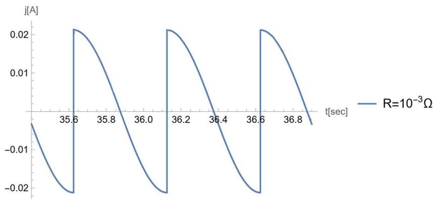
Fig. 14 The current profile for the case of negligible load. Parameters used are:  $C_s = 5 \times 10^{-2} \text{ F m}^{-2}$ ;  $S_T = 0.002 \text{ m}^2$ ;  $\varepsilon = 0.5$ ;  $\Theta_w = 0.5$ ;  $V_{\text{ref}} = 1.5 \text{ V}$ ;  $\eta = 6.3 \times 10^{-2} \text{ Pa s}^{-1}$ ;  $\gamma = 2.27 \text{ N m}^{-1}$ .
