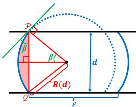
Fig. 12 Sketch of a droplet between two plates of separation  $d$  with consideration of a curved meniscus of curvature radius  $R$ . The wetting angle,  $\theta_w$  is related to the angle that subtends the arc,  $2\beta$ , by:  $\theta_w = \beta + \frac{\pi}{2} = \frac{1}{2}\theta_{\text{arc}} + \frac{\pi}{2}$ . The shaded region is a wedge trapped between the meniscus arc and the chord  $PQ$ .
