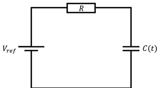
Fig. 1 Schematic of the electrical circuit and the principle of the reverse capacitive actuation. A time-varying capacitor  $C(t)$  is connected in series to a low-voltage battery,  $V_{\text{ref}}$  and an electric load,  $R$ . Varying the capacitance periodically, by using mechanical work, creates alternating current of electrons through the circuit.
