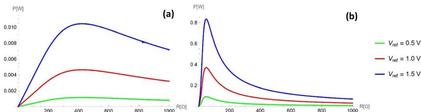
Fig. 10 Average power profile against the electric load for a porous electrode. Plotted for different stride frequencies at  $\omega = 2\pi \text{ s}^{-1}$  where the pore radius  $r_p$  is (a)  $10^{-5} \text{ m}$  and (b)  $10^{-7} \text{ m}$ . Other parameters used are:  $C_s = 5 \times 10^{-2} \text{ F m}^{-2}$ ;  $S_T = 0.002 \text{ m}^2$ ;  $\varepsilon = 0.5$ ;  $\theta_w = 131.18^\circ$ ;  $\eta = 6.3 \times 10^{-2} \text{ Pa s}^{-1}$ ;  $\gamma = 2.27 \times 10^{-2} \text{ N m}^{-1}$ .
