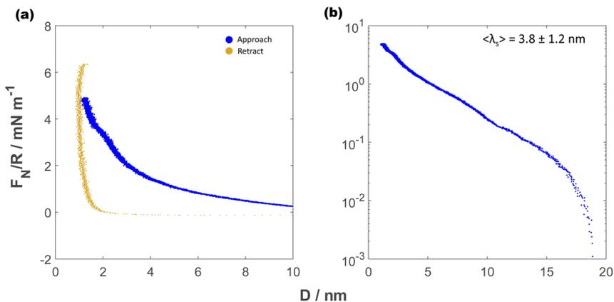
Fig. 5 Measurements of the normalised force between mica sheets as a function of separation,  $D$ , across 70 vol% EAN. (a) Linear scale forces at  $D < 10$  nm with retraction (gold) shown from the innermost layer. (b) Log–linear representation of normal force displaying long-range decay with average decay length of  $\langle \lambda_s \rangle = 3.8 \pm 1.2$  nm.
