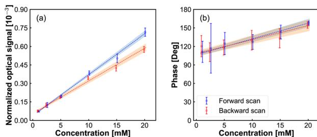
Fig. 4 Normalized optical amplitude (a) and phase (b) signals from lock-in amplifier vs.  $\text{Fe}(\text{MeOH})_2$  concentration. DC potential scan from  $-200$  mV to  $300$  mV with a scanning rate of  $40$   $\text{mV s}^{-1}$ , frequency of potential modulation is  $75$  Hz, the amplitude of potential modulation is  $50$  mV.
