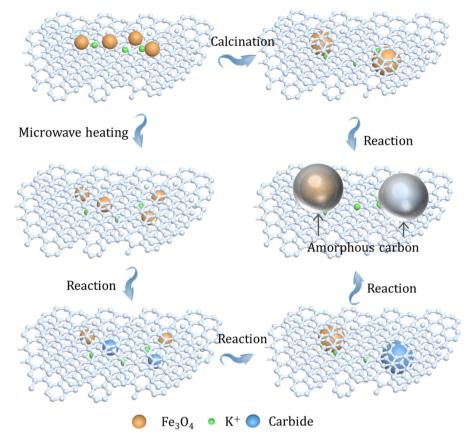
Fig. 5 Schematic diagram of the changes in active iron species microenvironment on different catalysts after high-temperature heating treatment and reaction.
