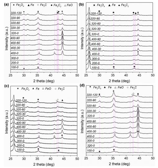
Fig. 2 In situ XRD patterns of different catalysts under given conditions: (a) K-Fe/AC-W-10, (b) K-Fe/CNF-W-10, (c) K-Fe/GA-W-10, and (d) K-Fe/ MPC-W-10. Notes: the reduction temperature was raised from room temperature to 400 °C and reduced for 90 min in a H<sub>2</sub> atmosphere, then the reaction gas was switched to reaction and phase changes were in situ detected. In terms of 320-120, 320 represents 320 °C and 120 stands for 120 min at 320 °C.
