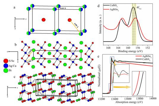
Fig. 5 Crystal structures of (a) AgBiS<sub>2</sub>, (b) AgBiSe<sub>2</sub> and (c) CuBiS<sub>2</sub>. Comparison of XPS spectra of Bi 4f (d) and XANES spectra of the Bi-L III edge (e) for AgBiSe<sub>2</sub> and CuBiS<sub>2</sub> electrocatalysts.
