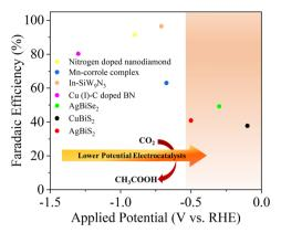
Fig. 1 Reported faradaic efficiency for the conversion of CO<sub>2</sub> to acetic acid as a function of applied potential on various catalysts. 12,44-46
