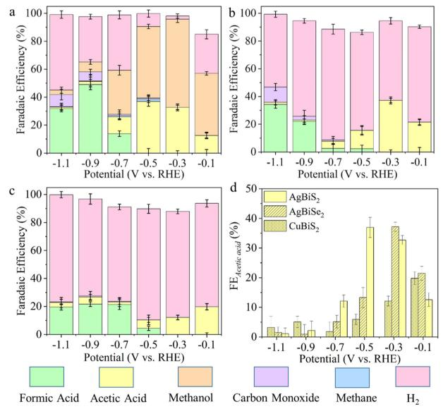
Fig. 2 Faradaic efficiency for each CO2 reduced gaseous product (carbon monoxide, methane, hydrogen) and major liquid product (methanol, formic acid and acetic acid) as a function of potential after 1 hour of CA during the eCO<sub>2</sub>RR on (a) AgBiS<sub>2</sub>, (b) AgBiSe<sub>2</sub> and (c) CuBiS<sub>2</sub>, and (d) comparison of FE for acetic acid at different potentials for all the catalysts.
