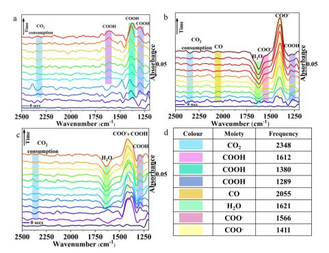
Fig. 3 (a-c) ATR-IR spectra during electrochemical CO<sub>2</sub> reduction on AgBiSe<sub>2</sub>, AgBiS<sub>2</sub>, and CuBiS<sub>2</sub> electrodes, respectively, at an applied potential of -0.1 V vs. RHE and (d) adsorption frequencies of different intermediates adsorbed on the catalyst surface during  ${
