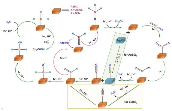
Fig. 4 Proposed reaction mechanism of the eCO<sub>2</sub>RR for the production of CH<sub>3</sub>COOH and HCOOH on CuBiS<sub>2</sub>, AgBiSe<sub>2</sub>, and AgBiSe<sub>2</sub> predicted from in situ IR experiments.
