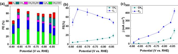
Fig. 1 (a) Product distribution during the CORR as a function of the applied potential on the CP-Cu<sub>0.812</sub> electrode. (b) FEs of C<sub>2</sub> and CH<sub>4</sub>. (c) The partial current density of C2 and CH4. The error bars represent the standard deviation from the measurements of three independent electrodes
