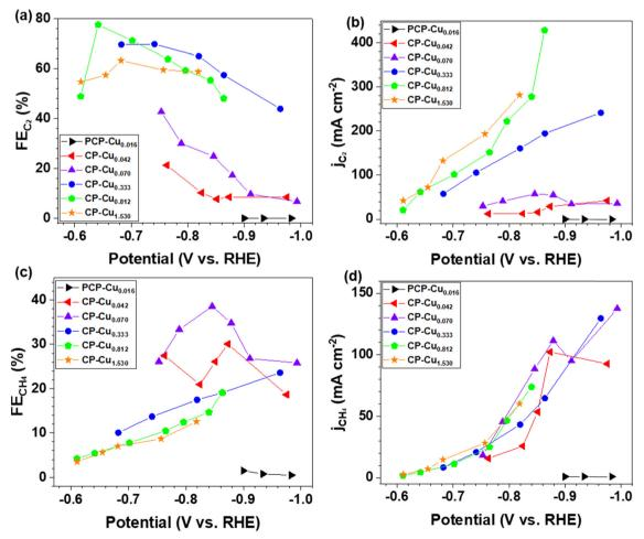
Fig. 2 (a) The partial current density and (b) FE of C2 during the CORR as a function of the applied potential using CP-Cu electrodes with various Cu loadings. (c) The partial current density and (d) FE of CH<sub>4</sub> as a function of the applied potential using CP-Cu electrodes with various Cu loadings.
