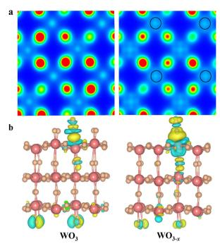
Fig. 1 (a) Distribution of charge density for the original WO<sub>3</sub> (left) and  $WO_{3-x}$  (right) plotted from 0 (blue) to 0.035 e<sup>-</sup> bohr<sup>-3</sup> (red). (b) Charge difference diagrams of \*CO adsorption on original WO<sub>3</sub> (left) and WO<sub>3-x</sub> (right); blue and yellow surfaces represent charge depletion and accumulation, respectively.
