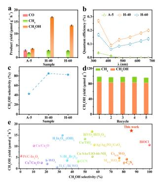
Fig. 3 (a) Product yields of the CO<sub>2</sub>RR using the different photocatalysts. (b) QE and (c) CH<sub>3</sub>OH selectivity values of different samples. (d) Photocatalytic stability of H-40 for five consecutive runs. (e) Comparison of CO<sub>2</sub>RR performance of WO<sub>3-x</sub> and other reported photocatalysts.
