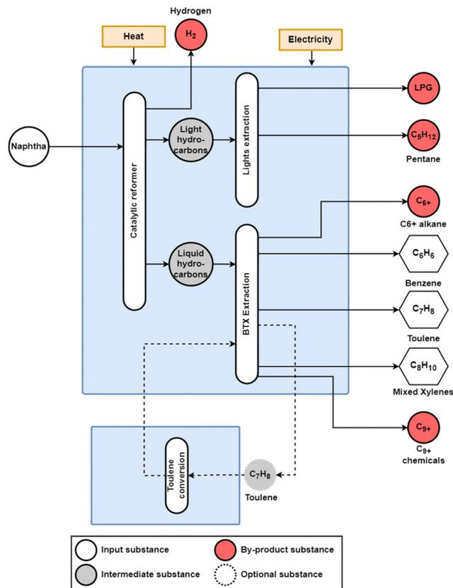
Fig. 4 Conventional naphtha catalytic reforming (CRR) process. The main products from this process are the BTX aromatics, and the by-products include pentane, C<sub>6+</sub> alkane, liquefied petroleum gas (LPG), and C<sub>9+</sub> chemicals, with an optional toluene conversion route to increase benzene and xylene yields. Adapted from Jiang *et al.*<sup>26</sup>
