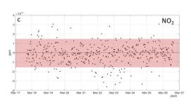
Fig. 4 Ten-day co-location data showing the difference between values measured in tube 2 minus tube 1. The expected difference for colocation would equal 0. Red shaded area denotes the  $\pm$  uncertainty assigned to each measurement. >90% of the data are included within the shaded area. (a)  $PM_{2.5} \pm 0.5 \ \mu g \ m^{-3}$ . (b)  $CO \pm 0.02 \ ppm$  (c)  $NO_2 \pm 0.0015 \ ppm$ .
