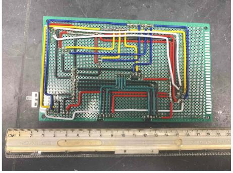
Fig. 2 (A) Photograph of sensor circuit board with components (a) plastic box, (b) Raspberry Pi computer, (c) PM<sub>2.5</sub> sensor, (d) A/D converter, (e) temperature and humidity recorder, (f) LED, (g) NO<sub>2</sub> sensor, (h) CO sensor. (B) Back of circuit board with wiring.
