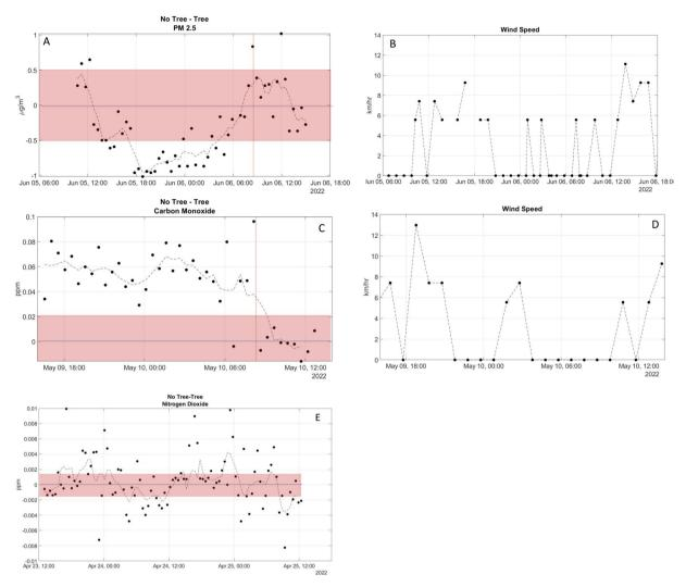
Fig. 6 (A) Difference between PM<sub>2.5</sub> in ambient air (tube 2) and tree canopy air (tube 1) vs. time. Tubes are co-located following the time indicated by the vertical red line. Dashed line is a 4-point running average. (B) Wind speed during the PM<sub>2.5</sub> experiment (C) same as (A) but for CO. (D) Wind speed during the CO experiment. (E) The difference between NO<sub>2</sub> in ambient and tree canopy air. Dashed line is a 4-point running average
