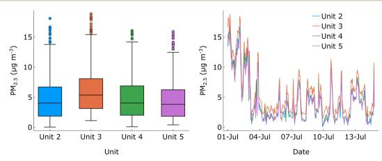
Fig. 2 Box plots and time series for uncorrected data from Units 2, 3, 4, and 5 obtained during the inter-unit sensor comparison period.
