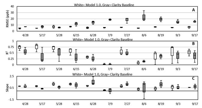
Fig. 4 Box and whisker plots for the (A) RMSE, (B)  $R^2$ , and (C) slope values of the Model 1.0 and Clarity baseline calibrated data from each 2 weeks collocation. Each point is a compilation of values from the 3 collocated sensors for that period. The lines within the boxes represent the medians, the interquartile range is the range of the boxes with the top representing the 75th and the bottom the 25th percentile. The whiskers represent the maximum and minimum values in the data.
