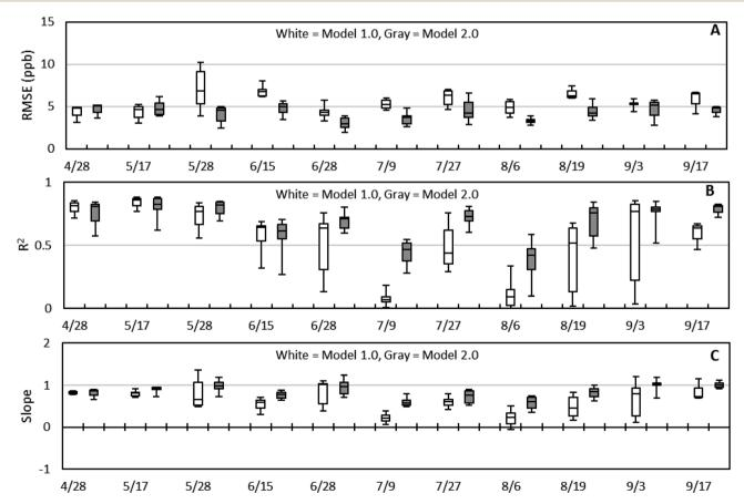
Fig. 9 Box and whisker plots for the (A) RMSE, (B)  $R^2$ , and (C) slope values of the Model 1.0 and Model 2.0 calibrated data from two-week periods. Each point is a compilation of values from the 3 sensors collocated during that date range. The lines within the boxes represent the medians, the interquartile range is the range of the boxes with the top representing the 75th and the bottom the 25th percentile. The whiskers represent the maximum and minimum values in the data.
