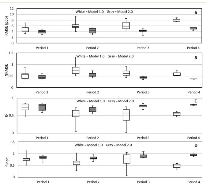
Fig. 8 Box and whisker plots for the (A) RMSE, (B) NRMSE, (C)  $R^2$ , and (D) slope values of the Model 1.0 and Model 2.0 calibrated data from each period. Each point is a compilation of values from the 12 sensors for that period. The lines within the boxes represent the medians, the interquartile range is the range of the boxes with the top representing the 75th and the bottom the 25th percentile. The whiskers represent the maximum and minimum values in the data.
