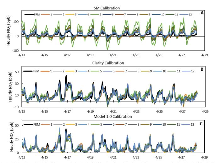
Fig. 3 (A) SM calibrated  $NO_2$  for all 12 sensors during the April 2021 collocation at West Phoenix. The average standard deviation is 10.3 ppb. (B) Clarity calibrated  $NO_2$  for all 12 sensors during the April 2021 collocation at West Phoenix. The average standard deviation is 1.66 ppb. (C)  $NO_2$  values using Model 1.0 for all 12 sensors during the April 2021 collocation at West Phoenix. The average standard deviation is 1.65 ppb.
