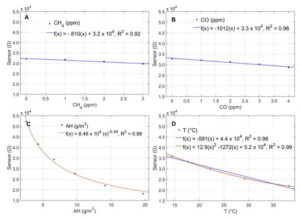
Fig. 2 Sensor response to (A) CH<sub>4</sub>, (B) CO, (C) AH, and (D) temperature in calibration chamber experiments.
