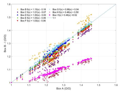
Fig. 1 Inter-sensor slope comparisons for 9 sensor boxes co-located in the laboratory over 8 consecutive days at 1 h resolution compared to Box A. For the purposes of comparison, sensor responses are normalized by their minimum observed values.
