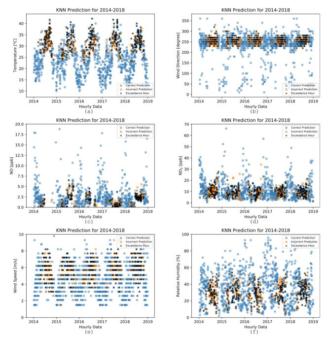
Fig. 11 Non-exceedance and exceedance hours for observed input variables: (a) temperature in °C, (b) wind direction in degrees, (c) NO in ppb, (d)  $NO_2$  in ppb,  $\in$  wind speed in m s<sup>-1</sup>, and relative humidity in%. Predictions were made using K-NN for the years 2014–2018 for Fontana using ONT meteorology. Hourly data from 12 PM to 5 PM are highlighted to reflect the peak ozone period.
