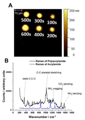
Fig. 2 For single-barrel SECCM eATRP of Am using [Am]: [HEBiB]: [Cu<sup>II</sup>]: [TPMA] = [20]: [1]: [0.5]: [0.625] at room temperature; (A) AFM image of the spots deposited at  $E_{\rm app} = -0.15$  V; (B) Raman spectrum of PAm deposited during an extended TOD experiment (TOD = 1800 s;  $E_{\rm app} = -0.15$  V). Raman settings-exposure time: 600 s, laser:  $\lambda$  = 820 nm, power: 100%, objective: 50×, grating: 1200 l mm<sup>-1</sup>, pinhole: IN.
