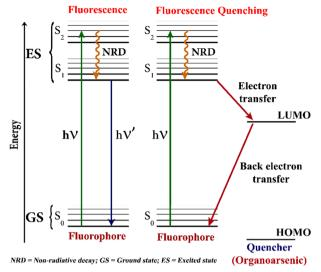
Fig. 2 A pictorial representation of the fluorescence guenching-based detection of organoarsenic feed additives using fluorescence chemosensors.
