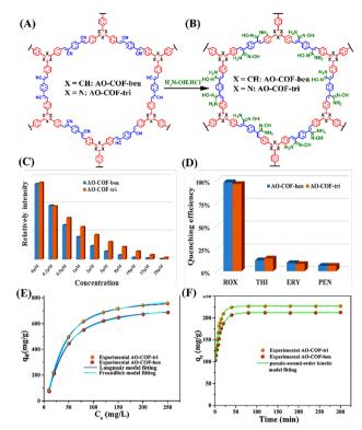
Fig. 10 The structures of functionalized COFs (A) AO-COF-ben and AO-COF-tri and (B) their post-functionalized structures; observed fluorescence changes after the addition of different concentrations of ROX to (C) AO-COF-ben and (D) AO-COF-tri; adsorption isotherms for ROX adsorption by (E) AO-COF-ben and AO-COF-tri; (F) adsorption kinetic curves of ROX by AO-COF-ben and AO-COF-tri. Reprinted with permission from ref. 80. Copyright 2022 Elsevier.
