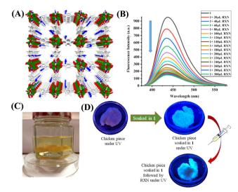
Fig. 8 (A) The 3D framework structure of luminescence Zn-MOF; (B) the changes in fluorescence emission spectra of Zn-MOF after adding increasing concentration of ROX (0-300  $\mu$ L); (C) chicken piece immersed in the solution of ROX; (D) colorimetric response of the chicken piece soaked in Zn-MOF and followed by the addition of ROX. Reprinted with permission from ref. 75. Copyright 2022 American Chemical Society.
