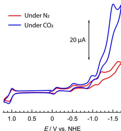
**Fig. 2** Cyclic voltammetry of **1** (1 mM) under  $\text{N}_2$  (red) or  $\text{CO}_2$  (Blue) in NMP, with 0.1 M  ${}^n\text{Bu}_4\text{NPF}_6$  supporting electrolyte vs. NHE redox couple. Glassy carbon working electrode ( $d = 3$  mm), Pt wire counter electrode, and a SCE reference (corrected to NHE, see ESI $^\dagger$ ).
