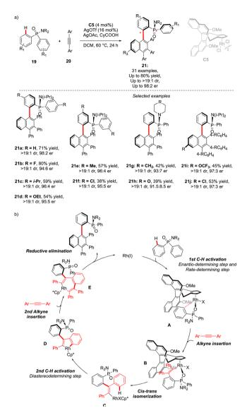
Scheme 8 Chiral CpXRh-catalyzed reaction delivering scaffolds featuring C-C atropoisomerism + P-point chirality via construction of the aromatic motif.
