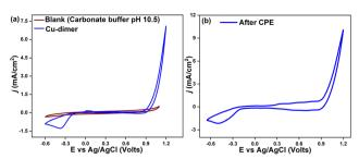
Fig. 3 (a) CV curves of 0.5 mM Cu-dimer in 0.08 M carbonate buffer (pH 10.5), scan rate 100 mV s $^{-1}$ . (b) CV curve of rinsed FTO after CPE in 0.08 M carbonate buffer (pH 10.5), at a scan rate of 100 mV s $^{-1}$ .
