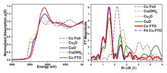
Fig. 5 (a) Normalized XANES spectra  $\mu(E)$  and (b) Fourier-Transform  $FT|k^3\chi(k)|$  spectra of the Cu deposit and reference oxides, and fitting to
