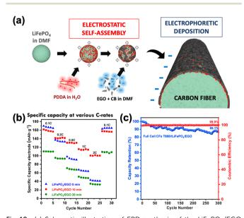
Fig. 10 (a) Schematic illustration of EPD synthesis of the LiFePO<sub>4</sub>/EGO electrode composite. (b) Specific capacities (normalized over the total mass of both electrodes, anode and cathode) at various C-rates. (c) Cycling performance and Coulombic efficiency at 1C. Reproduced with permission.<sup>6</sup> Copyright 2021, Elsevier.
