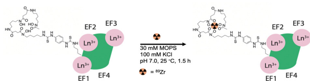
Fig. 3 Schematic description of no carrier-added radiochemical labeling procedure for the introduction of ^{89}\text{Zr} to the exogenous, DFO metal ion binding site of DFO-LanM.
