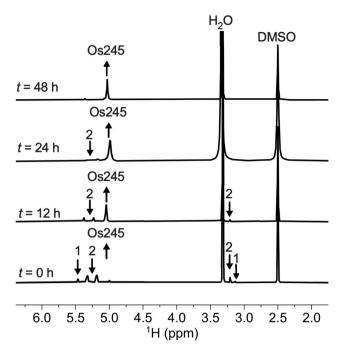
Fig. 1  $^{1}$ H NMR spectra (500 MHz, 25  $^{\circ}$ C, DMSO- $d_{6}$ ) showing the conversion of **1** and **2** to Os245 by heating in refluxing HCl. Arrows indicate the growth or disappearance of peaks.
