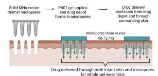
Fig. 1 Schematic of proposed poloxamer formulation application with microneedle pre-treatment. The formulation remains on the skin even after the micropores have closed, which permits ongoing drug delivery from a drug depot in the micropores as well as delivery through the surrounding intact skin. Figure made with Biorender.com.
