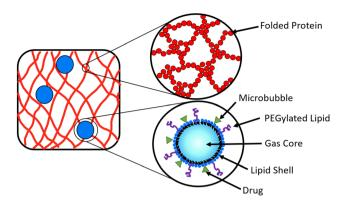
Fig. 2 Schematic depicting microbubbles (blue spheres) encompassed within a folded protein hydrogel network (red lines), where the hydrogel network is composed of cross-linked folded proteins (red spheres). The inset of the MB shows drug molecules (green triangle) attached to the lipid shell, where the lipid shell stabilises the gas core.
