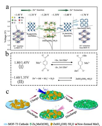
Fig. 5 (a and c) Schematic illustration of the Zn<sup>2+</sup> storage mechanism and (b) chemical reaction equation of the Zn<sup>2+</sup> insertion/extraction at different discharge/charge platforms of MOF-73 cathode
