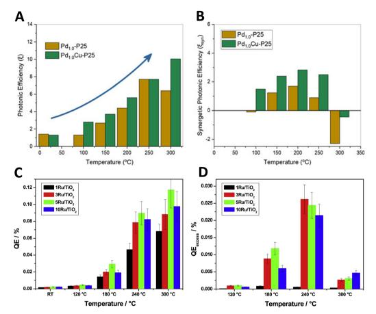
Fig. 4 Dark (thermo) and illuminated (thermo-photo) photonic-type efficiency as a function of temperature for hydrogen production using methanol:water mixtures. Bare (A) and excess (B) photonic yields of PdCu/TiO2 and reference catalysts. Reproduced with permission from ref. 55. Copyright Wiley. Bare (C) and excess (D) quantum efficiency (QE) for a series of Ru/TiO<sub>2</sub> catalysts. Reproduced with permission from ref. 40. Copyright Elsevier.
