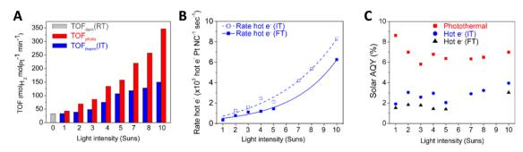
Fig. 5 TOF (A), excess reaction rate (B) and photonic yield (called the apparent quantum efficiency, AQE, (C)) vs. irradiance intensity for a Pt/TiO<sub>2</sub>/TiN catalyst. The excess function is called "Hot e". Observables are presented at two different temperatures (called IT, intermediate temperature, and FT, the final temperature of the reaction) in the panels. Reproduced with permission from ref. 56. Copyright ACS
