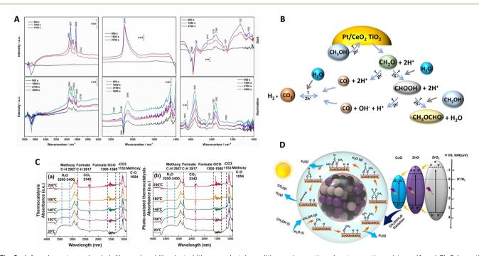
Fig. 6 Infrared spectra under dark (thermo) and illuminated (thermo-photo) conditions using methanol:water reaction mixtures (A and C). Schematic representation of the corresponding catalyst and catalytic process (B and D). Reproduced with permission from ref. 38 (Copyright Elsevier; panels A and B) and ref. 44 (Copyright Elsevier; panels C and D).
