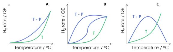
Fig. 3 Representative behaviors of the chemical (reaction rate) and photonic (quantum efficiency, QE) observables in thermal (T) and thermo-photo (TP) processes as a function of the reaction temperature.
