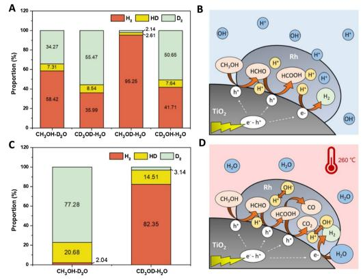
Fig. 7 Results from isotopic labelling experiments (A and C) and schematic process representation of the reaction mechanism (C and D) of a Ru/TiO<sub>2</sub> catalyst using a methanol:water mixture. Thermo (A and B) and thermo-photo (B and D) conditions are tested. Reproduced with permission from ref. 67. Copyright Elsevier.
